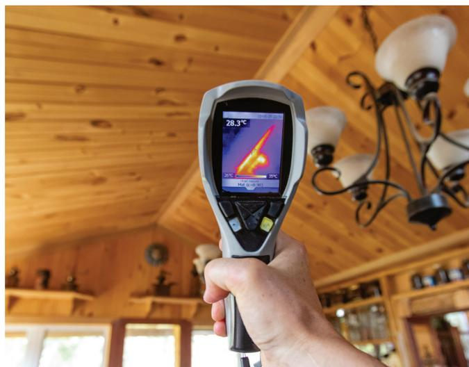
Some home inspections include technology that can detect where energy is lost and how a home's efficiency can be increased.
