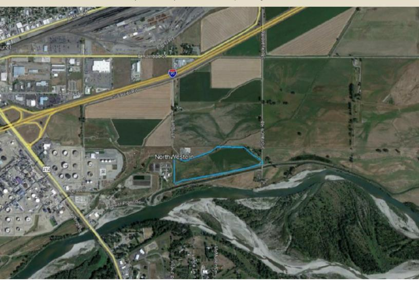
NorthWestern Energy proposes to build a 175-megawatt methane gas plant in Laurel on undeveloped land east of the CHS refinery, 300 feet from the Yellowstone River.
