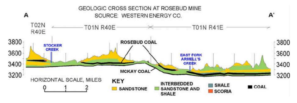
Figure 3. Cross sectional view of a portion of the Rosebud Mine (cross section location is shown in Figure 2.
